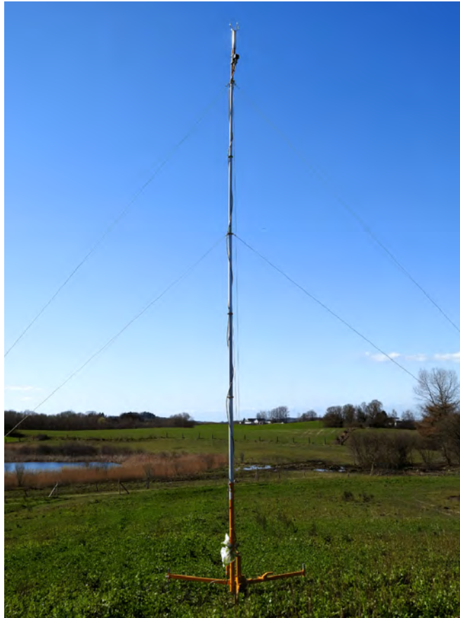
Figure 7.1: Picture of the extendable transportable mast. On top the Gill Ultrasonic Anemometer is placed.
