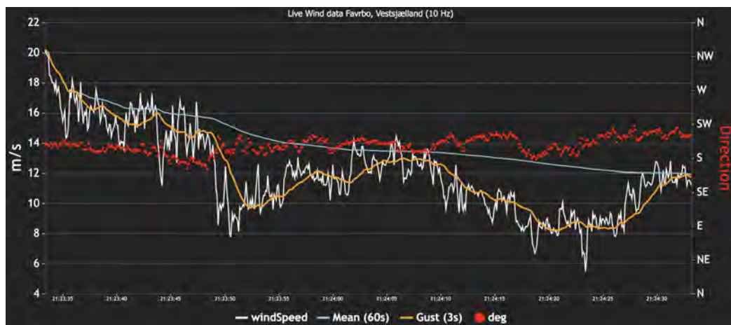
Figure 7.2: Real-time wind measurements from the web-application during one minute 7th February 2018 at 20:32:33 UTC to 20:33:33 UTC. The white curve shows the measured wind speed with a frequency of 10 Hz, given on the left axis. The orange and blue line shows the mean over 3 s and 60 s respectively. The red dots show the wind direction given on the right axis. On the internal webpage the plot updates with a frequency of 10 Hz.
