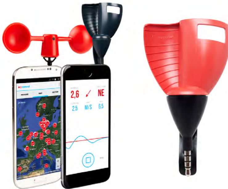
Figure 2.1: The Vaavud anemometers, Mjolnir (left) and Sleipnir (middle and right). The Sleipnir anemometer also measures the wind direction due to its asymmetric rotor design.
